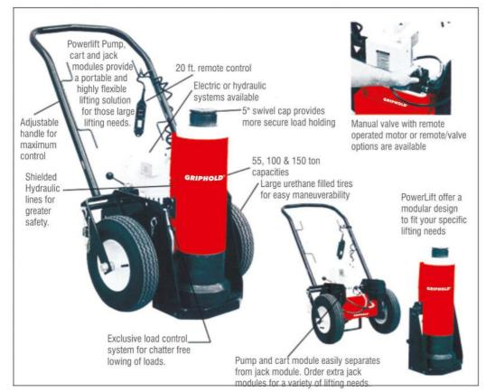
Modular design-pump and cart separates from cylinder and base.
